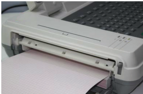
More than 10 kinds of printing methods, supporting Folded /Reel thermosensitive printing paper
